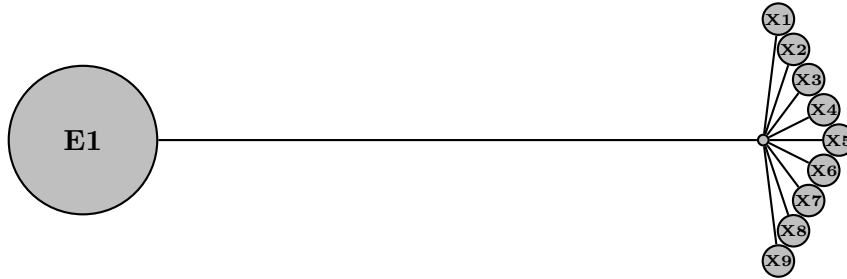
Figure 2: A gas network with one entry point and several exit points.
