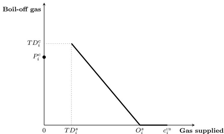
Figure 3: Boil-off consumption of a regasification plant.
